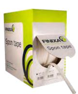
Round shaped foam strip for masking joints between two panels. One side of the strip has been treated with heat resistant adhesive. Simply stick the tape on the inside of one of the panels and close the other panel. 13mm and 25mm available.
