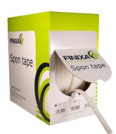
Round shaped foam strip for masking joints between two panels. One side of the strip has been treated with heat resistant adhesive. Simply stick the tape on the inside of one of the panels and close the other panel. 13mm and 25mm available.
