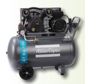
The latest in Atlas Copco's 3HP cast iron piston compressors. It is solid, robust and reliable. They are designed for professional applications where they offer trouble free performance even under demanding circumstances. Comes with a 100L tank and has a free dlivery of 190 litres/ min.
