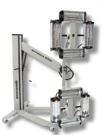
8x 1,000 watt infrared short wave lamps on 2 independently adjustable heads provide the maximum 3,081 sq. in.(2m²)cure area. Cure area is uniform and focused with no hot or cold spots. Each array of 4 lamps may be adjusted to conform to the contour of the panel.
